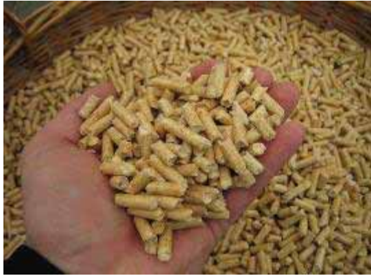
Figure 18: pellets & wood chips – fuels for automatic biomass installations; Source: NÖ Landwirtschaftskammer
