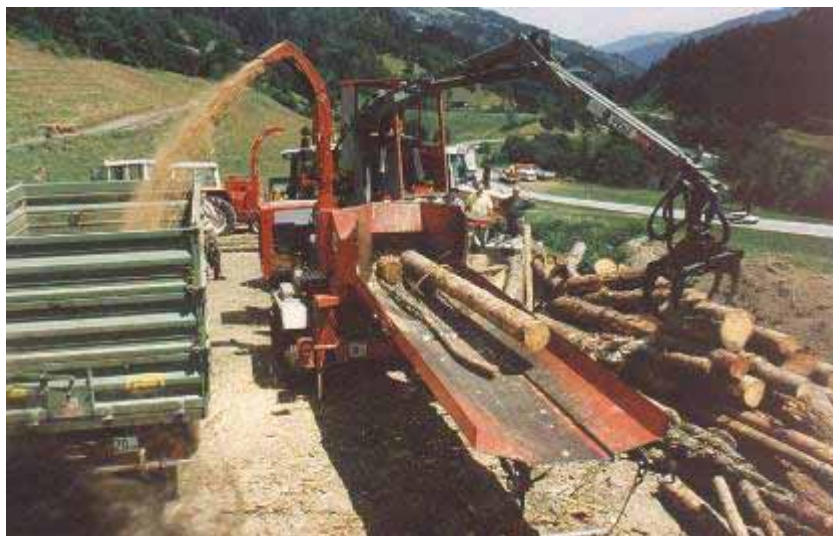
Figure 13: Wood chipper with mechanized feeding
