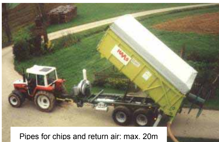
Figure 15: Wood chip delivery, standardized system with air blower
