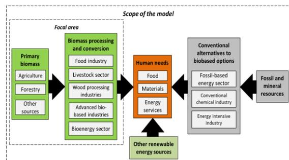
**Figure 2.** Schematic illustration of scope of the model and the focal area of the research
