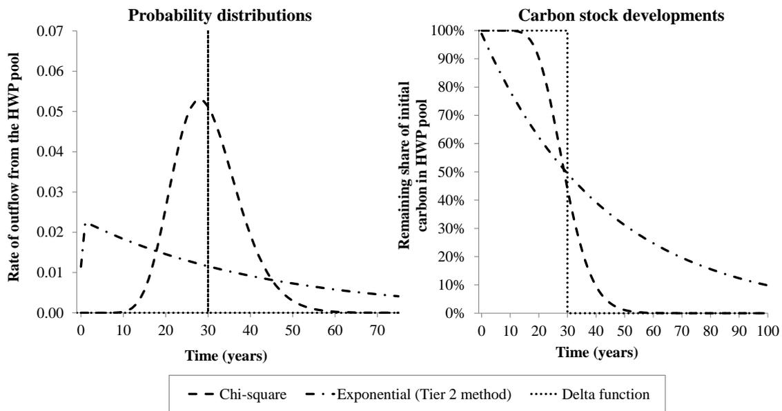
Figure 1. Probability distributions used to model carbon stock changes of wood products (left) and according carbon stock developments assuming a single inflow at  $t = 0$  (right)
