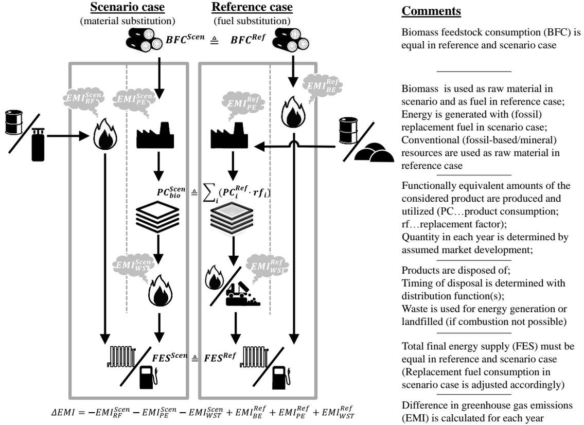
Figure 2. Schematic illustration of the model concept
