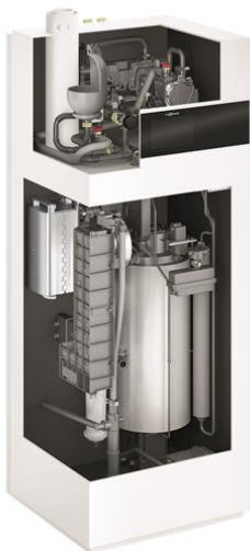
Fig. 6. Vitocalor PT 2 based on PEM-LT technology P_{el} : 750 W, P_{th} : 1,1 kW th P_{th} from gas boiler: individual scalable from 11,4 kW, 24,5 kW to 30,8 kW Hot water storage tank: 220 l
